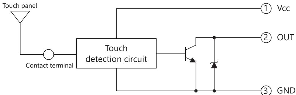
\*Because there is no reverse connection protection diode built-in, pay careful attention to the polarity of the power supply.
